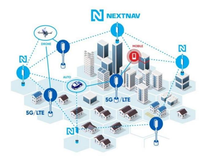
The TerraPoiNT beacons each include a high-precision atomic clocking source, and the ability to synchronize locally with nearby beacons by sharing their timing signals. The beacon network is also synchronized to Coordinated Universal Time, the global time standard broadcast by GPS and other NIST-traceable sources.
