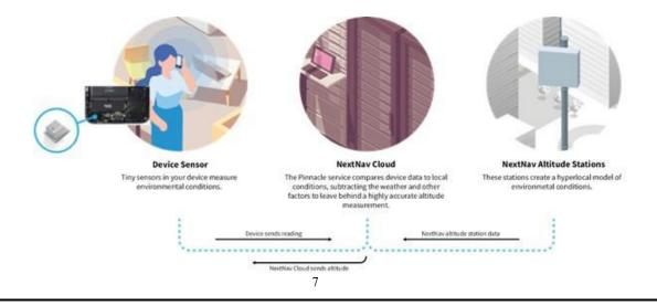
Pinnacle works by leveraging the physical principal that barometric pressure declines as altitude increases. By measuring the barometric pressure at a device, and comparing that measurement to the measurements from our network, we can accurately compute the altitude of the sensor. A Pinnacle altitude station is depicted below, and measures approximately 16" x 6" x 4".
